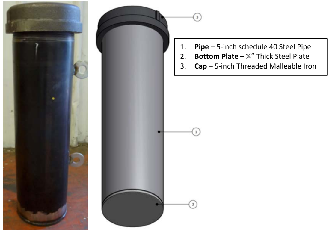
Fig. 3. High Capacity Versa-Pac 5-inch Pipe Container Design.
